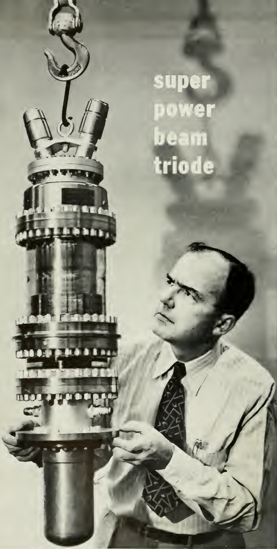
DR. L. P. GARNER OF THE LANCASTER, PA., PLANT EXAMINES ONE OF THE REMARKABLE 500-KILOWATT TUBES WHICH HE AND HIS ASSOCIATES DEVELOPED.
